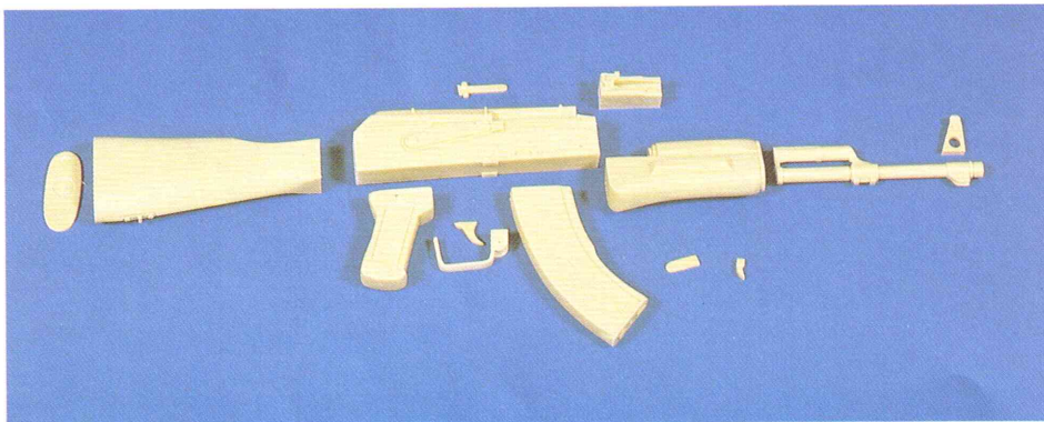
Resin parts after removing carrier and having been cleaned, ready to assemble.
