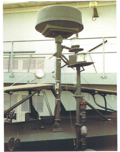
Fig.6 Close up of the radar and the top of the charthouse. Note the guys and stays.
