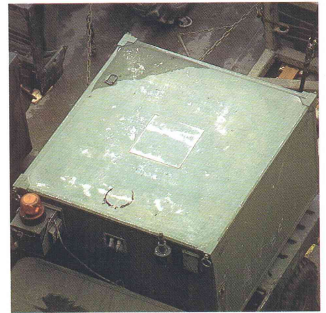
Fig.5 An overhead view to reveal upper deck detail. The square in the middle of the roof probably serves as an escape hatch.
