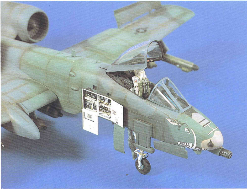
Fig. 4 The ACES II ejection seat and detail to the right. Note canopy linkage arms aft of the seat.
