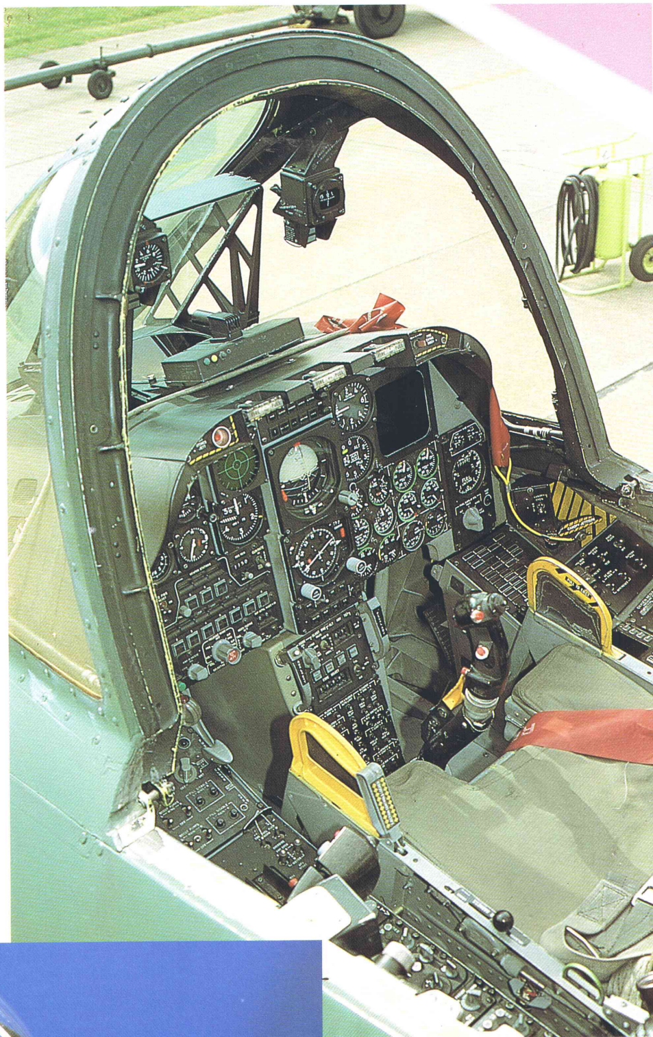
Fig. 7 Main instrument panel and the control stick in the A-10. Don't forget to add the stand-by compass to the windscreen frame.
